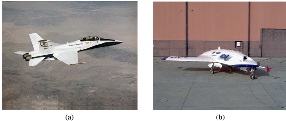
Figure 1.6: Military aerospace systems. (a) The F-18 aircraft is one of the first production military fighters to use “fly-by-wire” technology. (b) The X-45 (UCAV) unmanned aerial vehicle is capable of autonomous flight, using inertial measurement sensors and the global positioning system (GPS) to monitor its position relative to a desired trajectory. Photographs courtesy of NASA Dryden Flight Research Center.
