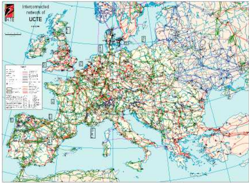
Figure 1.5: The European Power Network. By 2007 the European power suppliers will operate a single interconnected network covering a region from the Arctic to the Mediterranean and from the Atlantic to the Ural. In 2004 the installed power was more than 700 GW ( 7 \times 10^{11} W).
