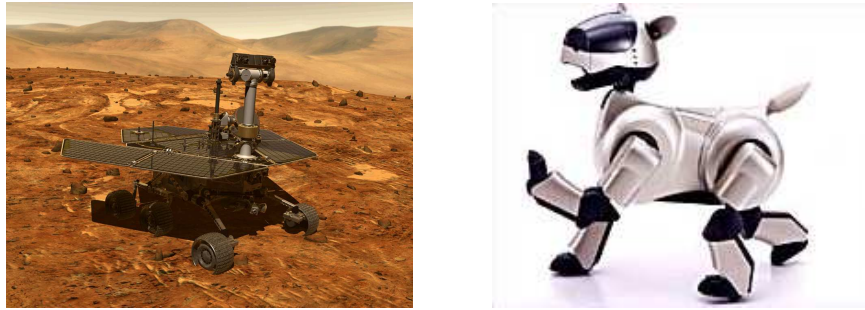
Figure 1.9: Robotic systems. (a) “Spirit”, one of the two Mars Exploratory Rovers that landed on the Mars in January 2004. (b) The Sony AIBO Entertainment Robot, one of the first entertainment robots to be mass marketed. Both robots make use of feedback between sensors, actuators and computation to function in unknown environments. Photographs courtesy of Jet Propulsion Laboratory and Sony.
